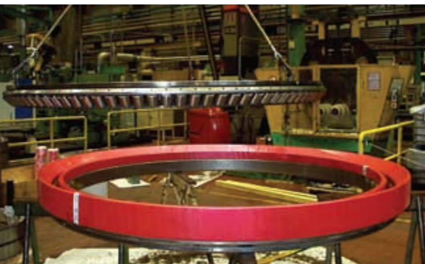
Placing a newly refurbished inner ring in a prepacked outer ring of a large bearing at FIS' repair centre in Wuppertal, Germany
